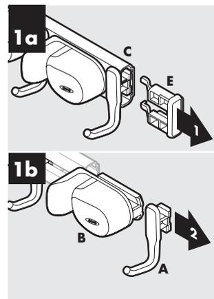
**1a.** To adjust configuration of the grip locks (**B**) and hooks (**A**), remove cap (**E**) on the right side of the organizer rail (**C**).
